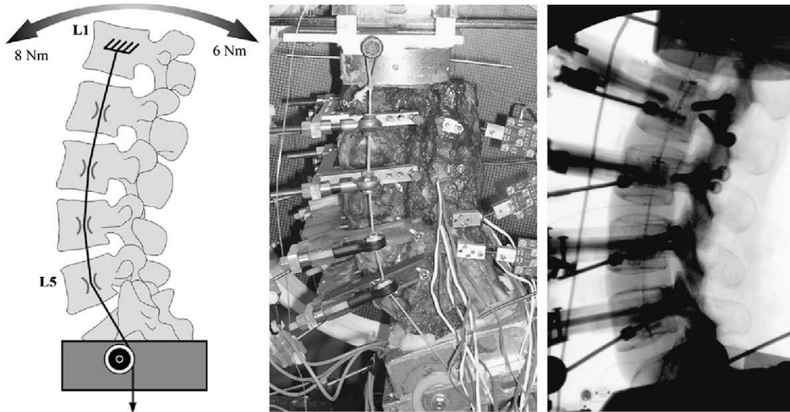
Fig. 1. Experimental set-up. (Left) Schematic; (Center) specimen photo; (Right) lateral X-ray.
