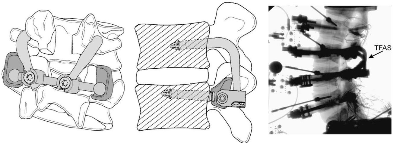
Fig. 2. Total Facet Arthroplasty System (TFAS) lumbar facet prosthesis. Artist's rendition of TFAS implanted in single functional spinal unit; (Left) posterior view; (Center) lateral cross sectional view; (Right) lateral fluoroscopic image of a test specimen implanted with TFAS (denoted by arrow).
