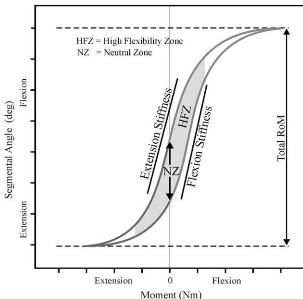
Fig. 3. Analysis of load-displacement curves in flexion-extension. The following parameters were quantified: 1) stiffness (slope of load-displacement curve) in the high-flexibility zone in flexion and extension (Nm/degree) and 2) neutral zone (degrees).
