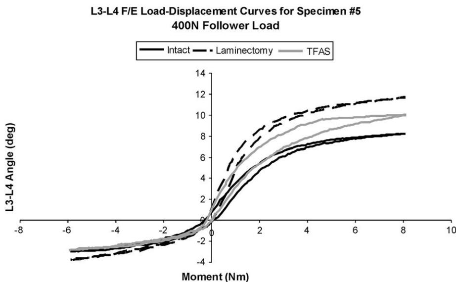
Fig. 4. Load-displacement curves for an L3–L4 segment in flexion-extension under 400 N preload. Intact, after complete L3 laminectomy and facetectomy, and after Total Facet Arthroplasty System implantation.
